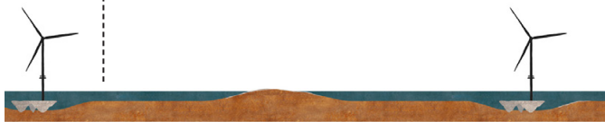
South west Doggerland The Grotto method will be used in places with an average depth of 20 metres.
