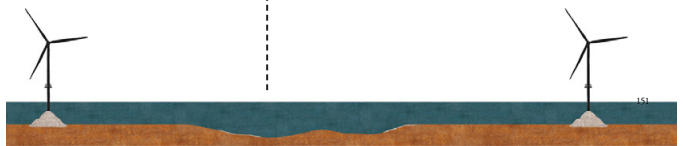
North east Doggerland The Cone method will be used in places with an average depth of 40 metres.
